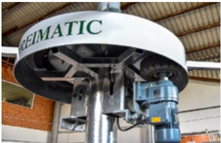
Drive system for tower horse walker
