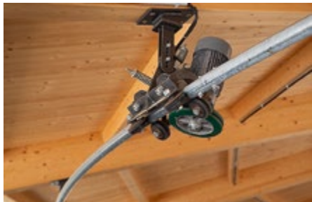
Drive system for round ring horse walker
